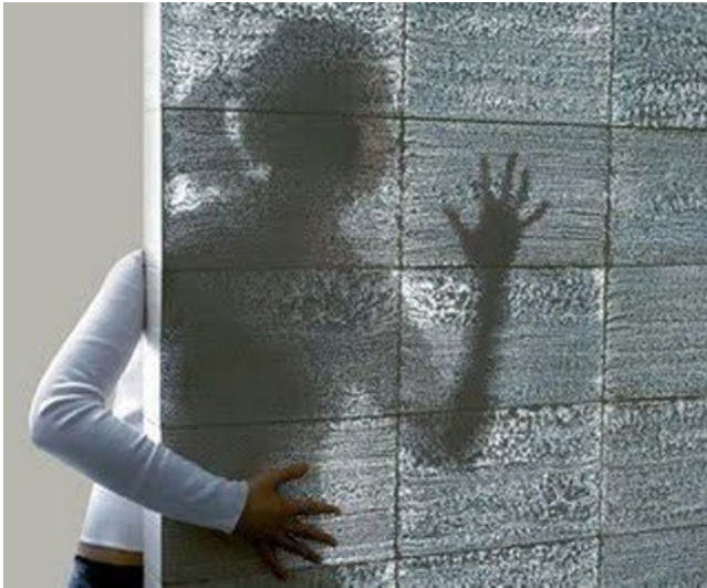
Figure 1. Transparent concrete wall ( http://theconstructor.org/concrete )
