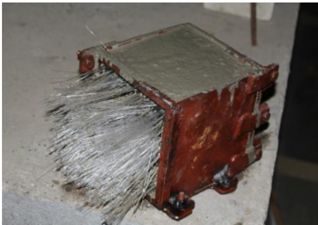
Figure 5. Casting of concrete blocks
